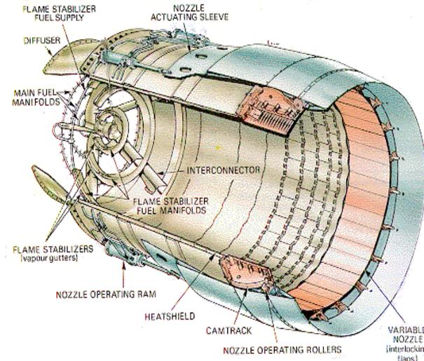
*Fig. 7. Cross-section of after burner*
