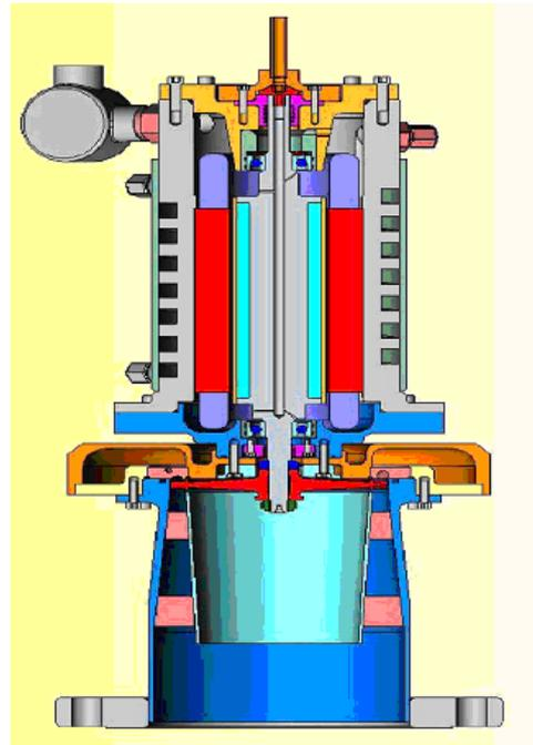
Fig. 6. Cross-section of turbo starter
