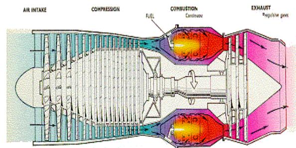
**Fig. 1.** *A turbojet engine*
