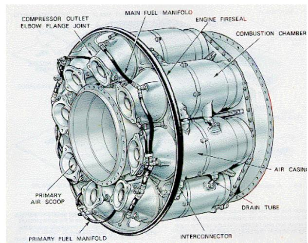
*Fig. 4. Combustion chamber*
