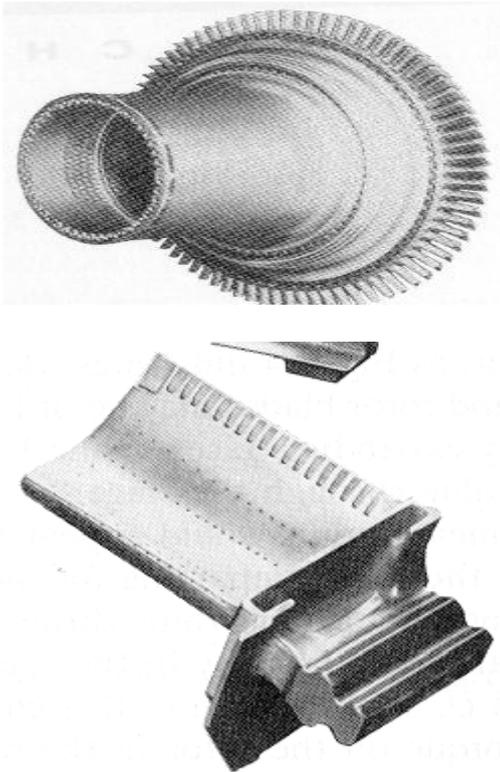
Fig. 5. HP-Turbine and a turbine blade
