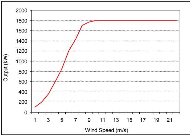
**Fig 2** Power Curve of Wind Turbine (V90)
